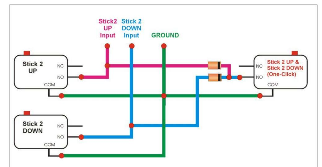
This method allows the button on the right to activate the Joystick 2 UP and Down Inputs simultaneously.
